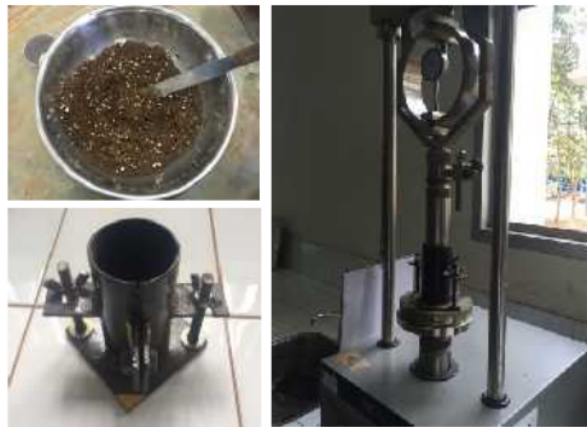
Figure 4. Specimens made by static compaction
