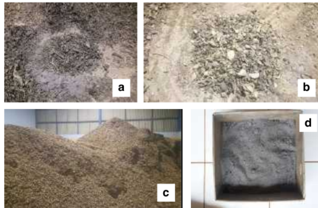
Figure 2. POTFA production process. (a) tea leaves, (b) palm oil shell, (c) mixing of palm oil and tea leaves, (d) Combustion residue as the palm oil-tea fuel ash (POTFA) .
